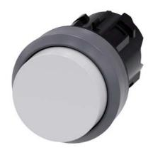
Pushbutton, 22 mm, round, plastic with metal front ring, white, pushbutton, raised momentary contact type, with laser labeling, upper case and lower case, always upper case at the beginning of the word
