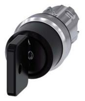
Key-operated switch O.M.R, 22 mm, round, metal, shiny, lock number 73034, black, with 2 keys, 3 switch positions I-O-II, latching, actuating angle 2x45°, 10:30h/12h/13:30h, key removal O, Z=50-unit packaging
