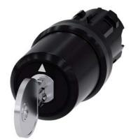
Key-operated switch BKS, 22 mm, round, plastic, lock number S1, with 2 keys, 3 switch positions I>O<II, momentary contact on the left, latching on the right, actuating angle 2x45°, 10:30h/12h/13:30h, key removal O, with laser labeling, upper case and lower case, always upper case at the beginning of the word
