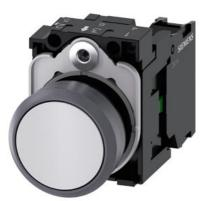
Pushbutton, 22 mm, round, plastic with metal front ring, white, pushbutton, flat, momentary contact type, with holder, 1 NO, screw terminal, Z=20-unit packaging
