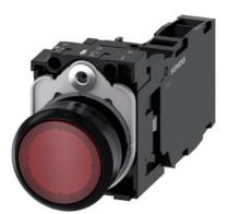
Illuminated pushbutton, 22 mm, round, plastic, red, pushbutton, flat, momentary contact type, with holder, 1 NO+1 NC, LED module with integrated LED 24 V AC/DC, screw terminal, with laser labeling, symbol number according to, ISO 7000 or IEC 60417
