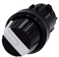
Selector switch, 22 mm, round, plastic, white, Rotary knob, 4 switch positions I-II-III-IV, latching, Actuating angle  $4x90^\circ$ , 3h/6h/9h/12h, with laser labeling, lower case
