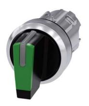
Selector switch, illuminable, 22 mm, round, metal, shiny, green, selector switch, short, 3 switch positions I-O<II, left latching, right momentary contact type, actuating angle 2x45°, 10:30h/12h/13:30h, Z=50-unit packaging
