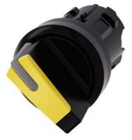
Selector switch, illuminable, 22 mm, round, plastic, yellow, selector switch, short, 2 switch positions O<I, momentary contact type, Actuating angle 45°, 10:30h/12h, with laser labeling, upper case
