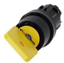
Key-operated switch O.M.R, 22 mm, round, plastic, lock number 73033, yellow, with 2 keys, 2 switch positions O-I, latching, actuating angle 90°, 10:30h/13:30h, Key removal O+I Z=50-unit packaging
