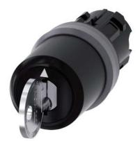
Key-operated switch IKON, 22 mm, round, plastic with metal front ring, lock number 360012K1, with 2 keys, 3 switch positions I>O<II, momentary contact type, actuating angle 2x45°, 10:30h/12h/13:30h, key removal O, with laser labeling, upper case and lower case, always upper case at the beginning of the word
