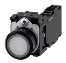
Pushbutton, 22 mm, round, plastic, clear, pushbutton, flat, momentary contact type, with holder 1 NO+1 NC, screw terminal, with laser labeling, inscription or symbol Customer-specific selection with SIRIUS ACT configurator (CIN)
