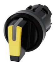
Selector switch, illuminable, 22 mm, round, plastic, yellow, selector switch, short, 3 switch positions I-O-II, latching, actuating angle 2x45°, 10:30h/12h/13:30h, with laser labeling, inscription or symbol Customer-specific selection with SIRIUS ACT configurator (CIN)
