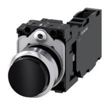
Pushbutton, 22 mm, round, metal, shiny, black, pushbutton, raised, momentary contact type, with holder, 1 NO+1 NC, screw terminal, with laser labeling, upper case and lower case, always upper case at beginning of line
