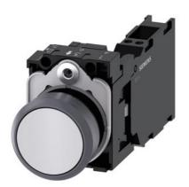
Pushbutton, 22 mm, round, plastic with metal front ring, white, pushbutton, flat, momentary contact type, with holder, 1 NO+1 NC, spring-type terminal, with laser labeling, upper case and lower case, always upper case at beginning of line
