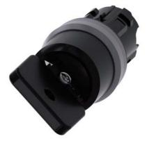
Key-operated switch O.M.R, 22 mm, round, plastic with metal front ring, lock number 73034, black, with 2 keys, 2 switch positions O-I, latching, actuating angle 90°, 10:30h/13:30h, key removal O+I, with laser labeling, upper case and lower case, always upper case at the beginning of the word
