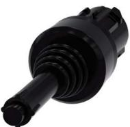
Coordinate switch, 22 mm, round, plastic, black, 2 switch positions, horizontal, momentary contact type, with mechanical interlocking, with laser labeling, upper case and lower case, always upper case at the beginning of the word
