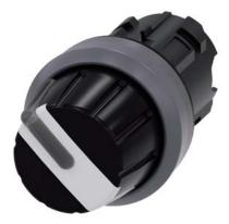
Selector switch, illuminable, 22 mm, round, plastic with metal front ring, white, Rotary knob, 2 switch positions O-I, latching, actuating angle 90°, 10:30h/13:30h, with laser labeling, lower case
