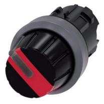
Selector switch, illuminable, 22 mm, round, plastic with metal front ring, red, Rotary knob, 2 switch positions O-I, latching, actuating angle 90°, 10:30h/13:30h, with laser labeling, upper case and lower case, always upper case at beginning of line
