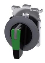
Selector switch, illuminable, 30 mm, round, Metal, matte, green, selector switch, long, front ring for flush installation, 3 switch positions I>O<II, momentary contact type, actuating angle 2x45°, 10:30h/12h/13:30h, with laser labeling, upper case and lower case, always upper case at the beginning of the word
