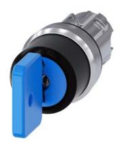
Key-operated switch O.M.R, 22 mm, round, metal, shiny, lock number 73038, blue, with 2 keys, 3 switch positions I-O-II, latching, actuating angle 2x45°, 10:30h/12h/13:30h, Key removal I+O+II, with laser labeling, upper case
