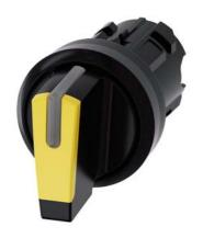
Selector switch, illuminable, 22 mm, round, plastic, yellow, selector switch, short, 3 switch positions I>O<II, momentary contact type, actuating angle 2x45°, 10:30h/12h/13:30h Z=50-unit packaging
