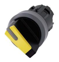
Selector switch, illuminable, 22 mm, round, plastic with metal front ring, yellow, selector switch, short, 2 switch positions O-I, latching, actuating angle 90°, 10:30h/13:30h, with laser labeling, lower case
