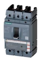
circuit breaker 3VA5 UL frame 250 breaking capacity class C 100kA @ 480V 3-pole, line protection TM230, FTAM, In=100A overload protection Ir=100A fixed short-circuit protection Ii=5...10 x In without connection
