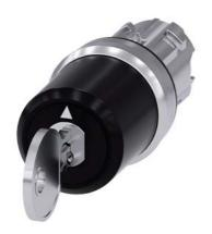
key-operated switch Siemens, 22 mm, round, metal, shiny, lock number SSG10, with 2 keys, 3 switch positions I-O-II, latching, actuating angle  $2x45^\circ,\,10:30h/12h/13:30h,$  key removal II, Z=50-unit packaging
