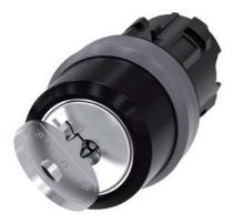
RONIS key-operated switch, 22 mm, round, plastic with metal front ring, lock number 455, with 2 keys, 2 switch positions O<I, momentary contact type, Actuating angle 45°, 10:30h/12h, key removal O, with laser labeling, upper case and lower case, always upper case at beginning of line
