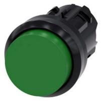
Pushbutton, 22 mm, round, plastic, green, pushbutton, raised, momentary contact type, with laser labeling, symbol number according to, ISO 7000 or IEC 60417
