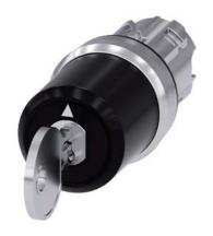
key-operated switch Siemens, 22 mm, round, metal, shiny, lock number SSG10, with 2 keys, 3 switch positions I-O-II, latching, actuating angle  $2x45^{\circ}$ , 10:30h/12h/13:30h, key removal O, with laser labeling, lower case
