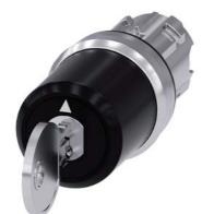
Key-operated switch BKS, 22 mm, round, metal, shiny, lock number S1, with 2 keys, 3 switch positions I>O<II, momentary contact type, actuating angle  $2x45^{\circ}$ , 10:30h/12h/13:30h, key removal O, with laser labeling, upper case and lower case, always upper case at the beginning of the word
