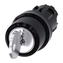
RONIS key-operated switch, 22 mm, round, plastic, lock number SB30, with 2 keys, 3 switch positions I>O<II, momentary contact on the left, latching on the right, actuating angle 2x45°, 10:30h/12h/13:30h, key removal O, possible special locks: SB31, 421, 455, with laser labeling, inscription or symbol Customer-specific selection with SIRIUS ACT configurator (CIN)
