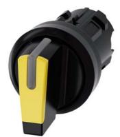
Selector switch, illuminable, 22 mm, round, plastic, yellow, selector switch, short, 3 switch positions I>O<II, momentary contact on the left, latching on the right, actuating angle  $2x45^{\circ}$ , 10:30h/12h/13:30h Z=50-unit packaging
