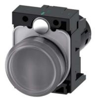
Indicator light with LED lamp, compact, 22 mm, round, plastic, clear with red-yellow-green LED, lens, smooth, with holder, operating voltage 6-24 V AC/DC, screw terminal, with laser labeling, symbol number according to ISO 7000 or IEC 60417
