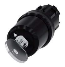
Key-operated switch BKS, 22 mm, round, plastic, lock number S1, with 2 keys, 2 switch positions O<I, momentary contact type, Actuating angle 45°, 10:30h/12h, key removal O, with laser labeling, lower case
