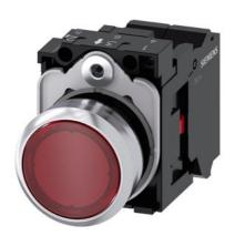
Illuminated pushbutton, 22 mm, round, Metal, shiny, red, pushbutton, flat, momentary contact type, with holder, 1 NC, LED module with integrated LED 230 V AC, spring-type terminal, with laser labeling, symbol number according to, ISO 7000 or IEC 60417
