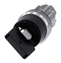
key-operated switch Siemens, 22 mm, round, metal, shiny, lock no. VL5, with 2 keys, 2 switch positions O<I, momentary contact type, actuating angle 45°, 10:30h/12h, key removal O, Z=50-unit packaging
