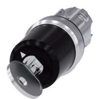
key-operated switch Siemens, 22 mm, round, metal, shiny, lock no. STGH10, with 2 keys, 2 switch positions O-I, latching, actuating angle 90°, 10:30h/13:30h, key removal O+I, Z=50-unit packaging
