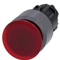
Illuminated mushroom pushbutton, 22 mm, round, plastic with metal front ring, red, 30 mm, latching, pull-to-unlatch mechanism, Z=50-unit packaging
