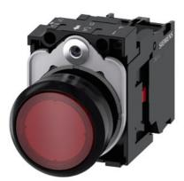
Illuminated pushbutton, 22 mm, round, plastic, red, pushbutton, flat, momentary contact type, with holder, 1NC, LED module with integrated LED 24 V AC/DC, screw terminal, with laser labeling, inscription or symbol Customer-specific selection with SIRIUS ACT configurator (CIN)
