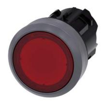
Illuminated pushbutton, 22 mm, round, plastic with metal front ring, red, pushbutton, flat, latching, Push-to-release mechanism, with laser labeling, upper case and lower case, always upper case at beginning of line
