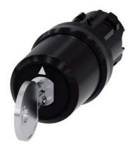
key-operated switch Siemens, 22 mm, round, plastic, lock number SSG10, with 2 keys, 3 switch positions I-O-II, latching, actuating angle 2x45°, 10:30h/12h/13:30h, key removal O+I, with laser labeling, upper case and lower case, always upper case at beginning of line
