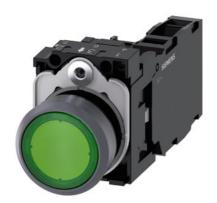
Illuminated pushbutton, 22 mm, round, plastic with metal front ring, green, pushbutton, flat, momentary contact type, with holder, 1 NO+1 NC, LED module with integrated LED 230 V AC, screw terminal, with laser labeling, symbol number according to, ISO 7000 or IEC 60417
