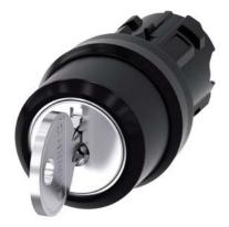
RONIS key-operated switch, 22 mm, round, plastic, special lock, with 2 keys, 3 switch positions I-O-II, latching, actuating angle 2x45°, 10:30h/12h/13:30h, Key removal II, possible special locks: SB31, 421, 455
