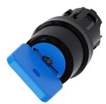
Key-operated switch O.M.R, 22 mm, round, plastic, lock number 73038, blue, with 2 keys, 2 switch positions O-I, latching, actuating angle 90°, 10:30h/13:30h, key removal O, with laser labeling, upper case
