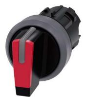
Selector switch, illuminable, 22 mm, round, plastic with metal front ring, red, selector switch, short, 3 switch positions I-O-II, latching, actuating angle 2x45°, 10:30h/12h/13:30h, with laser labeling, lower case
