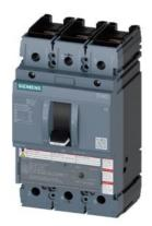
circuit breaker 3VA5 UL frame 250 breaking capacity class C 100kA @ 480 V 3-pole, line protection TM210, FTFM, In=70A overload protection Ir=70A fixed short-circuit protection Ii=10 x In UL489 SB (naval), 50 deg. cel. nut keeper kit on both sides
