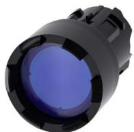
Illuminated pushbutton, 22 mm, round, plastic, blue, Front ring, raised, castellated, momentary contact type, with laser labeling, upper case and lower case, Always upper case at the beginning of the word
