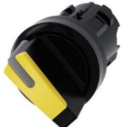
Selector switch, illuminable, 22 mm, round, plastic, yellow, selector switch, short, 2 switch positions O<I, momentary contact type, Actuating angle 45°, 10:30h/12h Z=50-unit packaging
