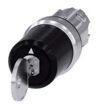
key-operated switch Siemens, 22 mm, round, metal, shiny, lock number SSG10, with 2 keys, 3 switch positions I>O<II, momentary contact on the left, latching on the right, actuating angle 2x45°, 10:30h/12h/13:30h, key removal II, Z=50-unit packaging
