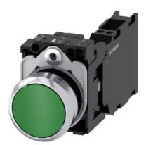
Pushbutton, 22 mm, round, metal, shiny, green, pushbutton, flat, momentary contact type, 1 NO+1 NC, spring-type terminal, with laser labeling, upper case
