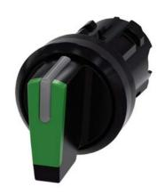
Selector switch, illuminable, 22 mm, round, plastic, green, selector switch, short, 3 switch positions I>O<II, momentary contact type, actuating angle 2x45°, 10:30h/12h/13:30h, with laser labeling, inscription or symbol Customer-specific selection with SIRIUS ACT configurator (CIN)
