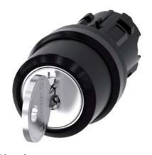
RONIS key-operated switch, 22 mm, round, plastic, lock number SB30, with 2 keys, 3 switch positions I-O<II, left latching, right momentary contact type, actuating angle 2x45°, 10:30h/12h/13:30h, key removal O, possible special locks: SB31, 421, 455, with laser labeling, upper case and lower case, always upper case at the beginning of the word
